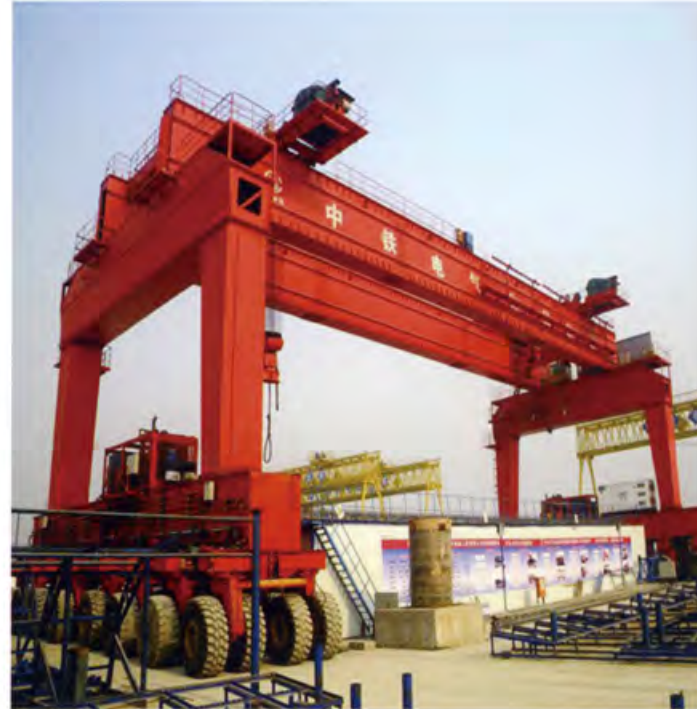
Rubber Tyred Girder Crane
